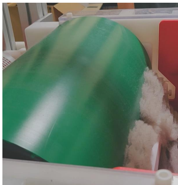
PET fibers are collected on electrodes
