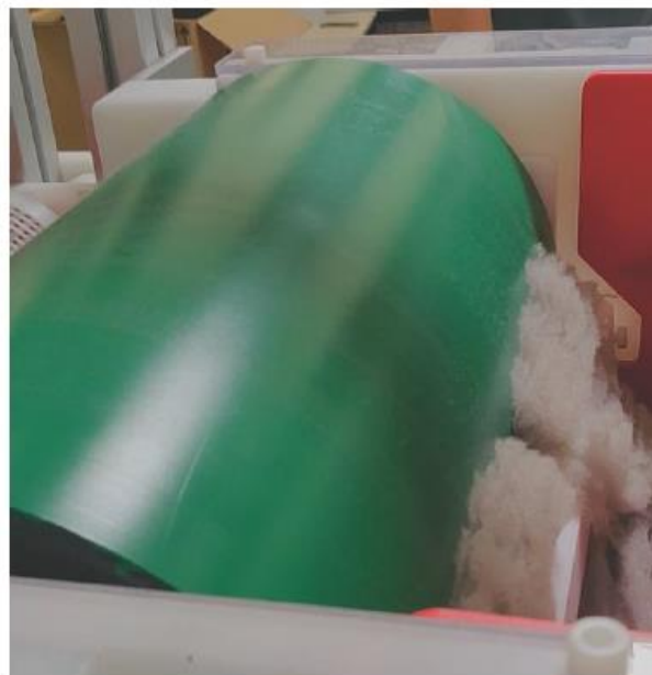
PET fibers are collected on electrodes
